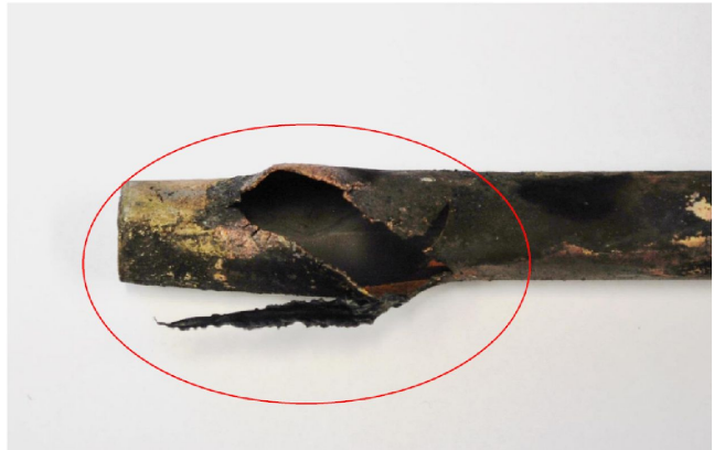
Pic2 Oxygen Pipe
